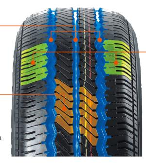
Small shoulder circumferential longitudinal grooves at both sides and plump little pattern blocks on shoulders bring indeal rigidity and excellent handing. meanwhile, small circumferentia longitudinal grooves enable tires shoulders to diffuse heat quickly, providing higher safety performance.
